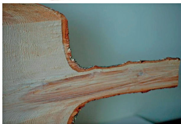
Fig. 1. Transverse and longitudinal section of a fir branch with visible dark heartwood (photo: Tadej Rejc).
