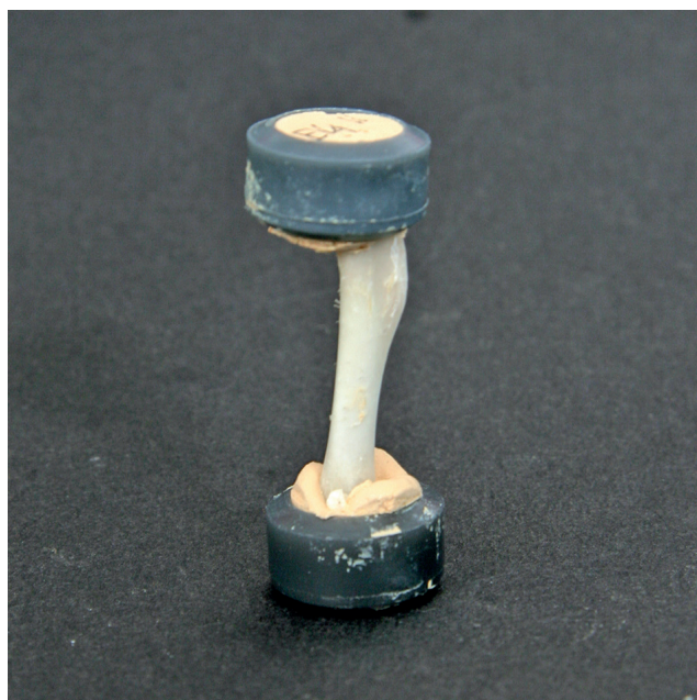
Fig. 2. Rat femur prepared for biomechanical bending test.
